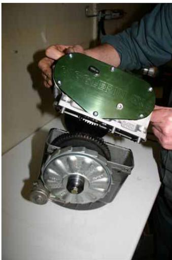
Apply a bead of silicone type sealant to the top housing and fit to the winch taking care that correct location and meshing is achieved.
