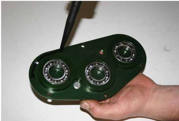
Apply a bead of silicone type sealant to the mating and fit side plate to the winch top housing.
