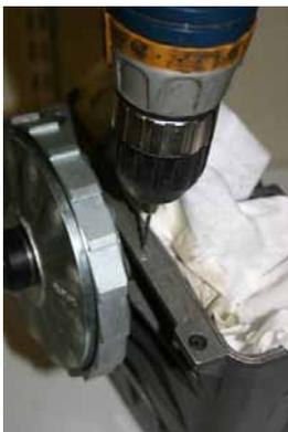
With the centre punch spot mark the centre of the scribe mark. Then make sure to protect the inside of the housing from swarf. Drill through the mark made by the punch with the 3.5mm drill bit. Then enlarge the hole with the 8mm drill bit. Clean away the swarf and tidy the edge of the new mounting hole.
