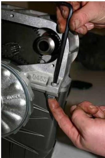
Without using sealant fit the new top housing to the winch taking care that it locates correctly.
