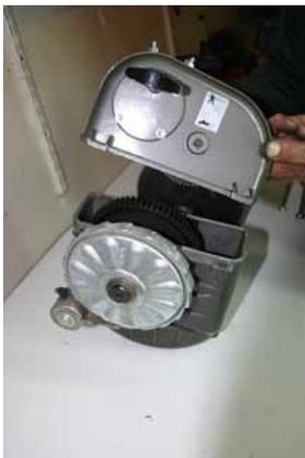
Using the ¼" Allen key, remove the 3 bolts that secure the upper motor housing and place to one side.
